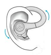
Place hook behind ear. Rotate and adjust for best fit.
