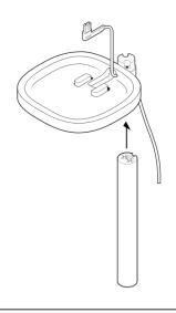
Use the 2 silver screws to attach the speaker platform to the top of the stem, threading the power cable carefully. Snap the bottom plate on with the power cable channel in the back, and mount the platform on the stem.
