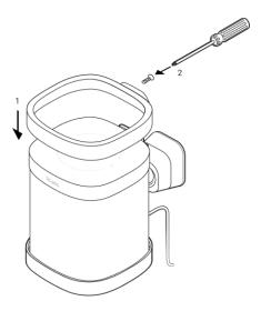
Slide the Mount down onto the wall bracket.
