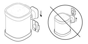
Twist the speaker to position it in place, then turn it right to lock it in securely.
