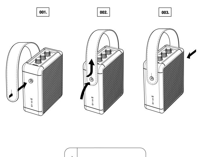
NOTE: ENSURE THAT THE CARRY STRAP IS SECURELY FASTENED ON BOTH SIDES BEFORE USE.
