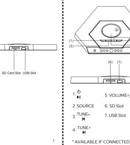
Press to turn on speaker.long press into stand-by. PLAY/PAUSE on the USB\*/SD\*/BT mode. 2. SOURCE:
