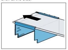
Tip: In order to avoid covering the inner ventilation opening (freezer compartment) during fitting, position the ice cube maker on the left-hand side of the fixed shelf.
