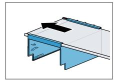
**Tip:** In order to avoid covering the inner ventilation opening (freezer compartment) during fitting, position the ice cube maker on the left-hand side of the fixed shelf.
