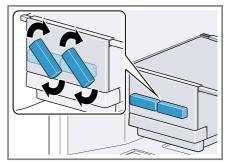
The ice cubes will loosen and fall into the ice cube container. **3.** Pull out the ice storage container and remove the ice cubes.
