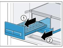
2. Lift the fixed shelf with the holder at the rear ① and remove it ②.
