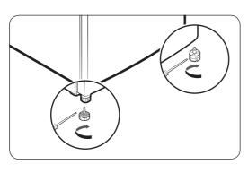
Level the refrigerator by manually adjusting the levelling feet. Turn the levelling feet clockwise to lower the position, or turn counter clockwise to raise.
