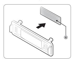
While holding the top and bottom sides of the filter case, unlock the filter case to reveal the **deodorizer filter (A)**. Replace the filter, and then reinsert the case.
