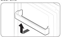
Slightly lift up and pull out the door bin.
