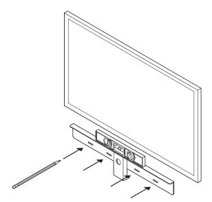
3. Use a 5/16" drill bit to drill pilot holes (see Wall mounting information)
