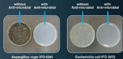
In tests conducted at the Mitsubishi Heavy Industries Nagoya Research Lab, 24 hrs after contact with bacteria, cultured on agar media.
