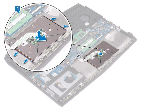
2 Replace the four screws (M2x2.5) that secure the touchpad to the palm-rest assembly.
