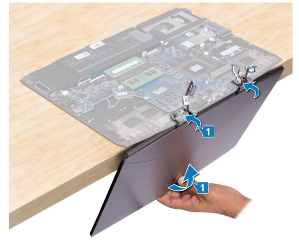
2 Replace the two screws (M2.5x2.5) that secures the hinges to the palm-rest assembly.
