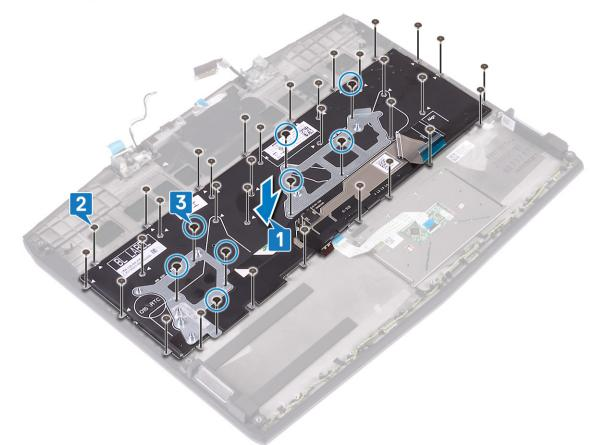
NOTE: The keyboard is shipped with a Mylar, that has to be adhered to the keyboard bracket after replacing the screws. Mylar has three layers: clear release paper, black Mylar, and blue Mylar.
