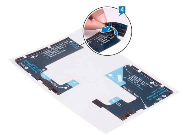
**5** Using the alignment holes, adhere the keyboard Mylar on the left side of the keyboard bracket.
