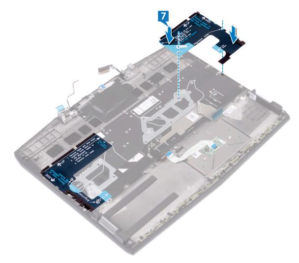
8 Peel the blue Mylar from both the sides.
