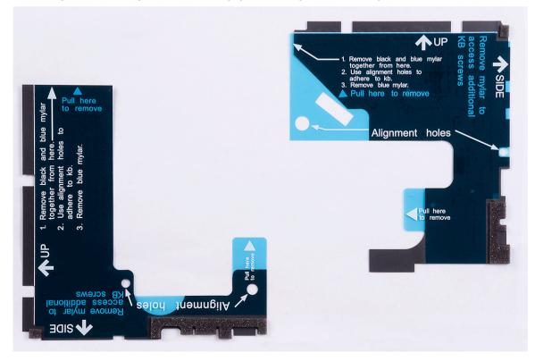
4 Peel the left black Mylar, along with the blue Mylar from the clear release paper.
