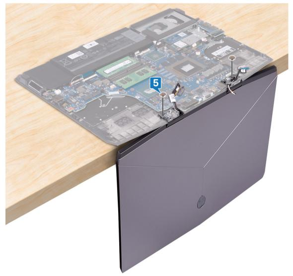
**6** Rotate the display assembly inward and lift up and away from the palm-rest assembly.
