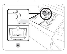
First insert the provided liquid detergent guide in the **II** main-wash compartment. Then, apply liquid detergent to the guide below the marked max line (A).
