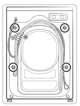
1. Locate the shipping bolts (marked with circle in the figure) on the rear side of the washing machine.
