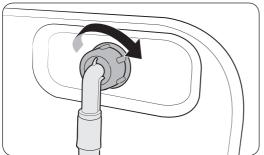
2. Connect the other end of the water hose to the inlet valve on the back of the washing machine. Turn the hose clockwise to tighten.
