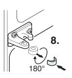
8. Remove hinge bushing, turn through 180° and re-fit.
