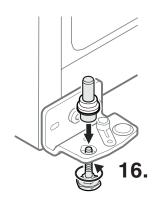
**16.** Tilt appliance slightly backwards, insert pin and attach using the adjustable foot.
