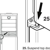
**25.** Suspend top door on hinge pin. For this, the door must be open at least 90°.
