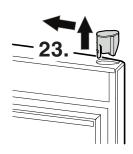
23. Using a screwdriver, push out the plug from underneath and transfer it to the opposite side.
