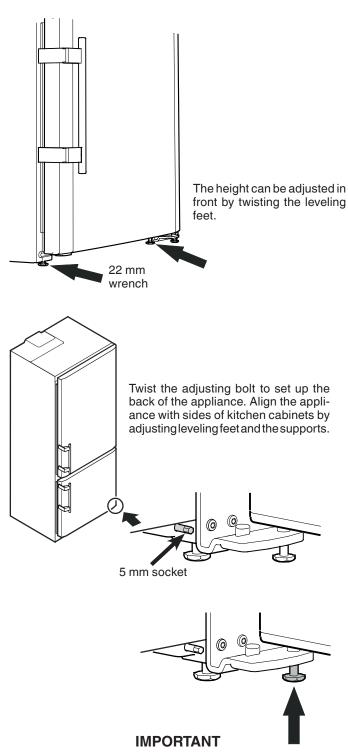
After final installation, this screw must be turned down until it has proper floor contact to support the hinge bracket.
