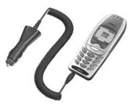
The input voltage range is from 11 to 32V DC, negative grounding. Avoid prolonged charging with the Rapid Mobile Charger (LCH–9) when the car engine is not running; this may cause the battery of your car to drain. In some cars the cigarette lighter plug is not provided with electricity if the ignition is not switched on.
